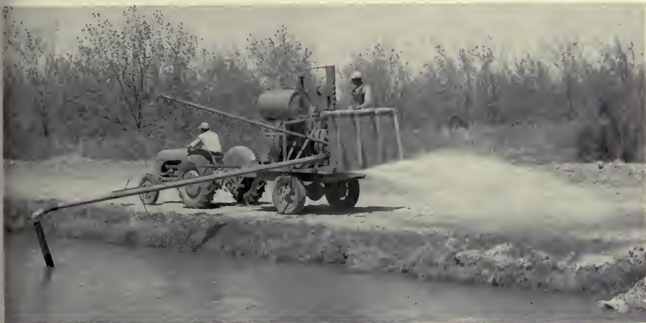
FOR LOCAL SPRINKLING use tractor trailer rig. Photo by Clarence Barsuk, Yuma County Water Users Association.
